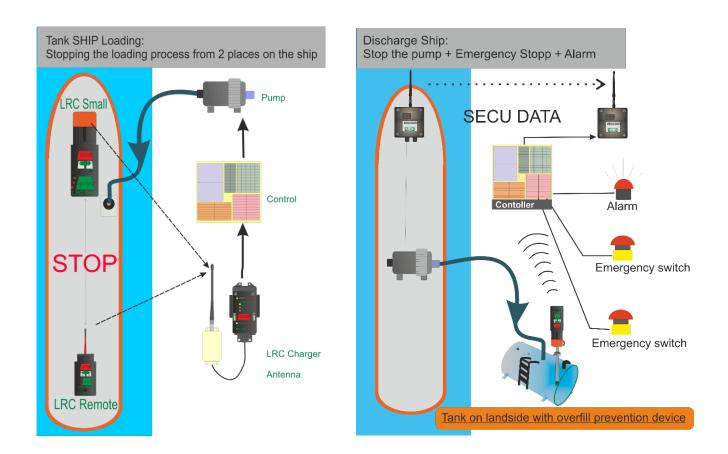
Secu-Tech offers an easy radio controlled sollution for the new ADNR 2007 regulation which demands an additional emergency stop on the schip during the ship loading and a stop-function for the shipspump during the unloading of the ship.
