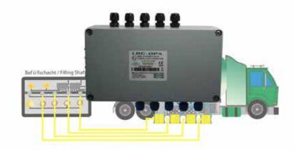
For delivery of Fuel Stations – supports PTC limit probes according to EN13616.
