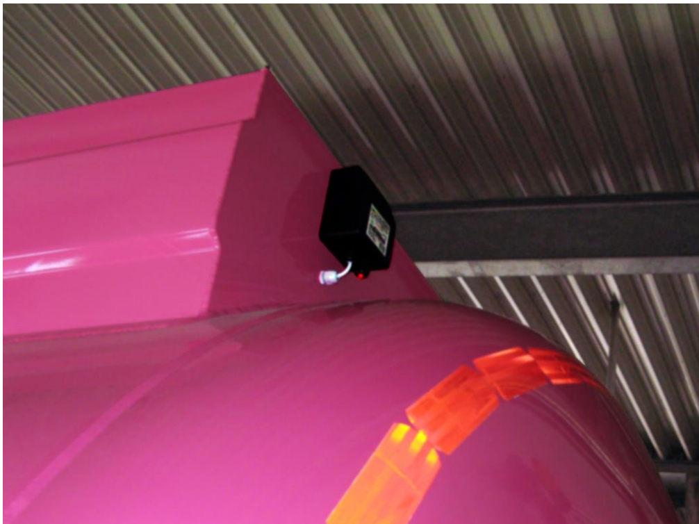
Practical example Installation of a SECU MultiGPS on a tank truck
